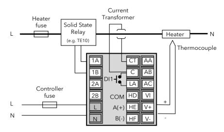
Note: a burden resistor value  $10 \boldsymbol{\Omega}$  is mounted inside the controller.
