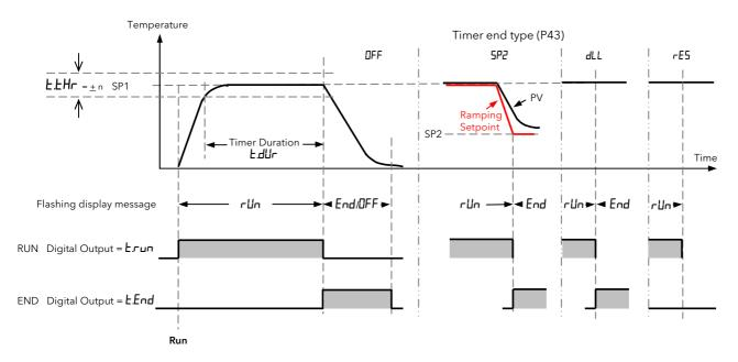
Notes: The dwell period can be reduced or increased while the timer is running by adjusting  $E_r E$  (Time Remaining) in Level 2.
