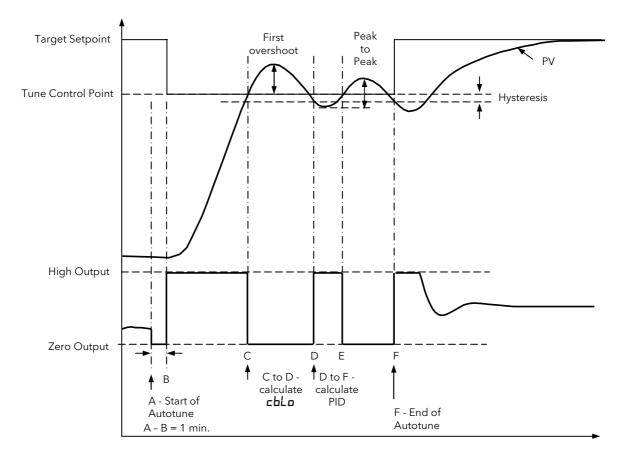
For a tune from below setpoint 'cbLa' is calculated on the basis of the size of the overshoot (assuming it was not set to Auto in the initial conditions).  $cbH_{i}$  is then set to the same value as cbLa.
