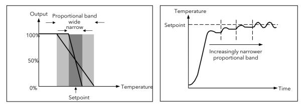
The diagram also shows the effect of narrowing proportional band to the point of oscillation. A very wide proportional band results in straight line control but with an appreciable initial error between setpoint and actual temperature. As the band is narrowed the temperature gets closer to setpoint. If the proportional band is very narrow the loop becomes unstable resulting in an oscillatory response.
