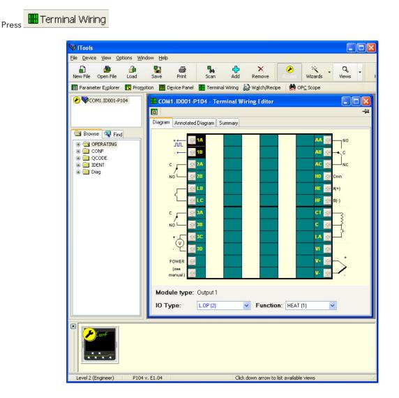
Click on the terminal numbers to show the type of output fitted and its function. The function can be changed using the drop down list. If no function is configured the small diagram showing connections on that output are removed.
