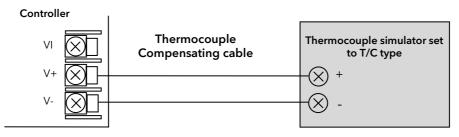
Set the mV source to the same thermocouple type as that configured in the controller.
