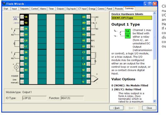
Click on the terminal numbers to show the I/O Type, Function and corresponding Help for that terminal. If no function is configured the small diagram showing connections on that output are removed.
