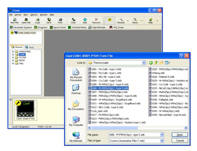
4. In this example a Pt-PTRh(10%) thermocouple has been loaded into the controller.
