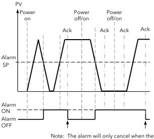
Note: The alarm will only cancel when the alarm condition is no longer current AND then it is acknowledged
