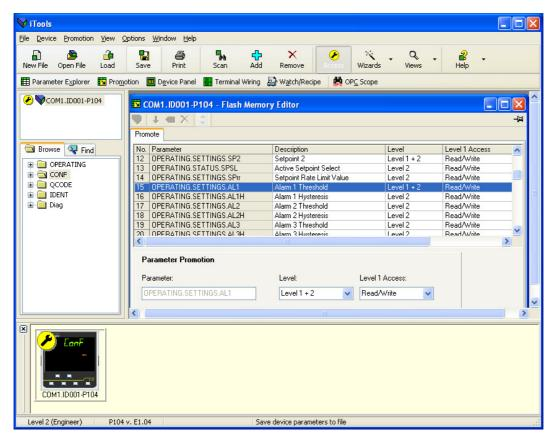
AL1 will now appear in the Level 1 list as well as the Level 2 list and will be read/write according to the selection in the above example.
