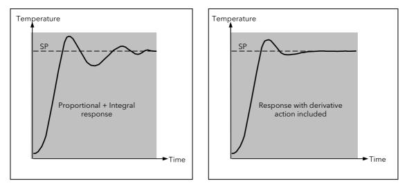
The derivative modifies the output to reduce the rate of change of error. It reacts to changes in the PV by changing the output to remove the transient. Increasing the derivative time will reduce the settling time of the loop after a transient change.
