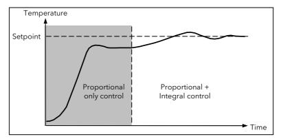
The units for the integral term are measured in time (1 to 9999 seconds). The longer the integral time constant, the more slowly the output is shifted and results in a sluggish response. Too small an integral time will cause the process to overshoot and even oscillate. The integral action may be disabled by setting its value to OFF.
