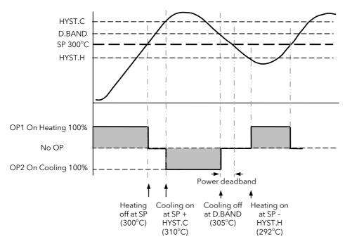
Example: Heating and Cooling Type both on/off Setpoint = 300°C Control Action = reverse Heating Hysteresis = 8°C Cooling Hysteresis = 10°C Deadband 50% of cooling hysteresis = 5°C
